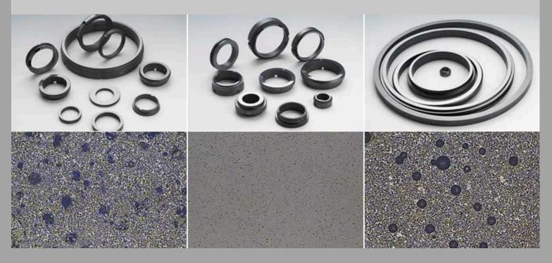
The phase diagram observed under a 200x optical microscope reveals that the distribution and size of the crystals in the pressure-free sintered silicon carbide material are consistent, with the largest crystal measuring no more than 10  $\mu$ m.
